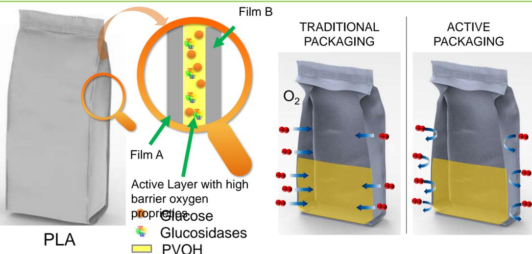
The oxygen scavenging activity is obtained by including in the multilayer film system a layer of glucose and glucosidases that catalyzes the oxygen absorption. Both the molecule and the enzyme are dissolved in a PVOH matrix and deposited on a PLA film, previously subjected to an appropriate plasma treatment in order to increase the film hydrophilicity.
